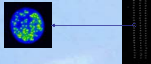
Figure 4. 10 nL THB cell array on a microscope slide
